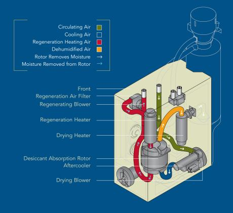
Matsui's desiccant rotor technology has become the industry standard in dehumidifying hot air drying equipment. Its unique, honeycomb design—molecular sieve desiccant, bonded and then baked onto ceramic paper—eliminates powder that can contaminate the system. Its large contact area effectively absorbs at high temperatures, drying resin in half the time while stabilizing dew points at a constant  $-40^{\circ}$ F.
