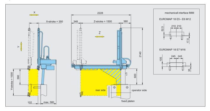
The special features of the REMAK handling system RX 32 are:
