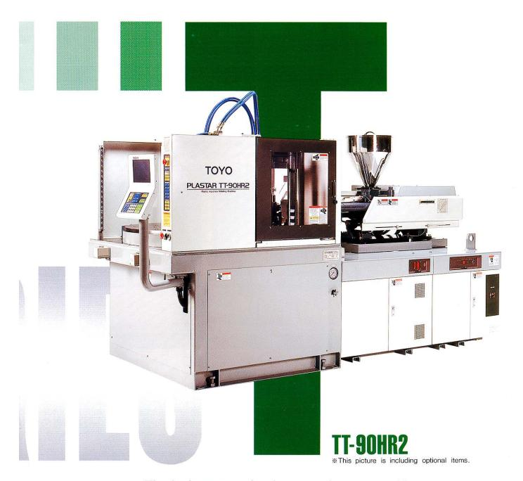
The basic construction is two-station rotary table with a horizontal injection unit. The clamping mechanism is hydraulic with three tie-bar structure.
